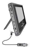
Connect the car adapter to a well accessible 12V cigarette lighter jack or 12V vehicle power supply output jack. The car adapter LED lights up red during operation.
